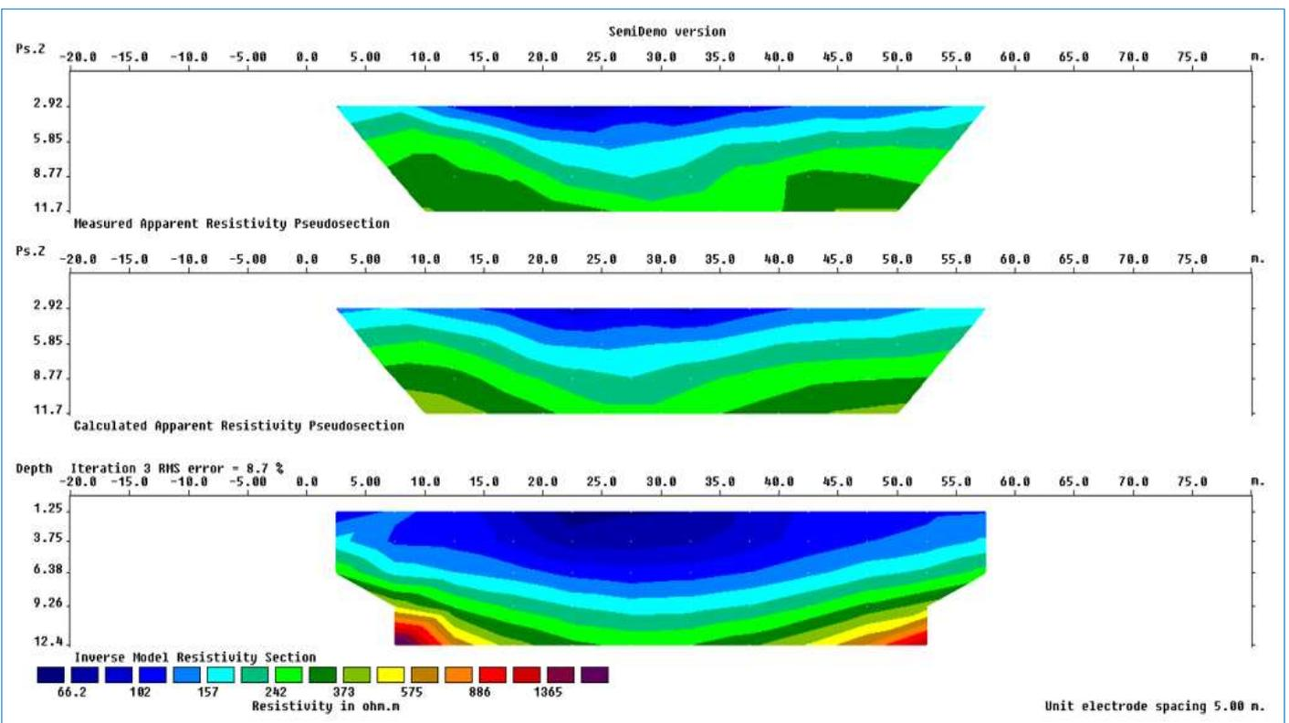
Fig. 9. Lateral Resistivity Profiling along Traverse One
