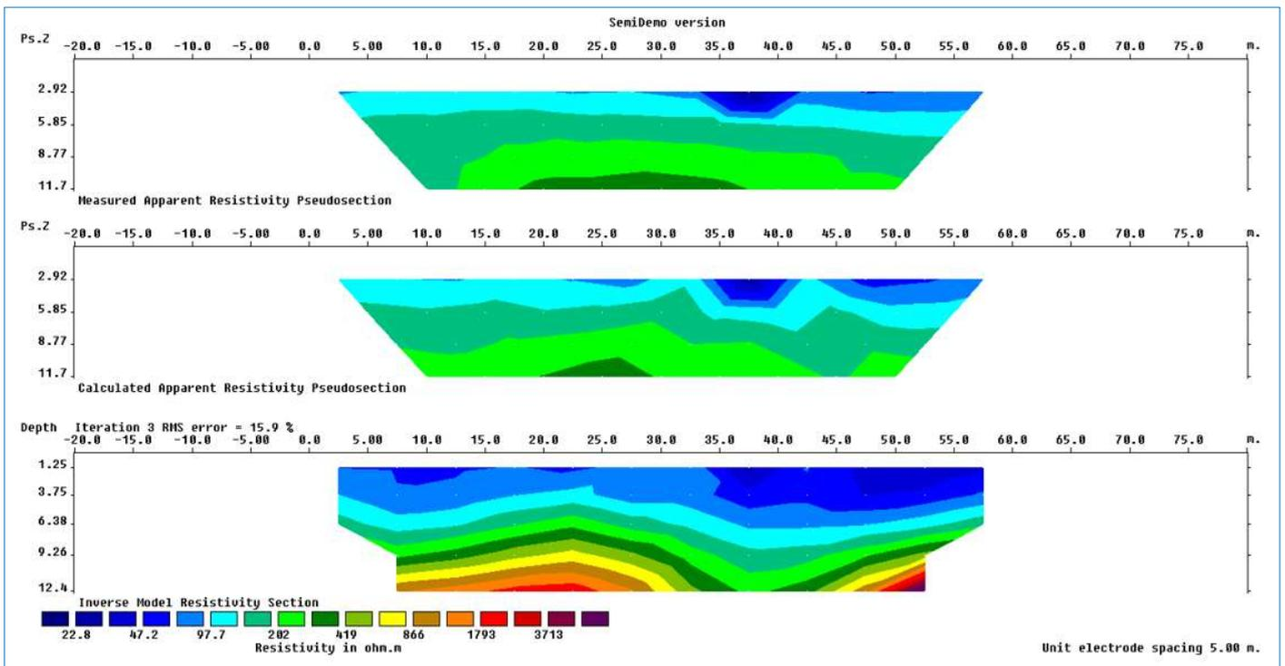
Fig. 9. Lateral Resistivity Profiling along Traverse Three
