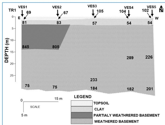
Fig. 12. Geoelectric section along Traverse One
