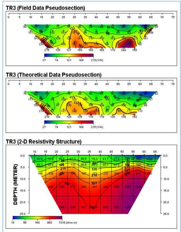
Fig. 8. Dipole-Dipole Pseudosection along Traverse Three
