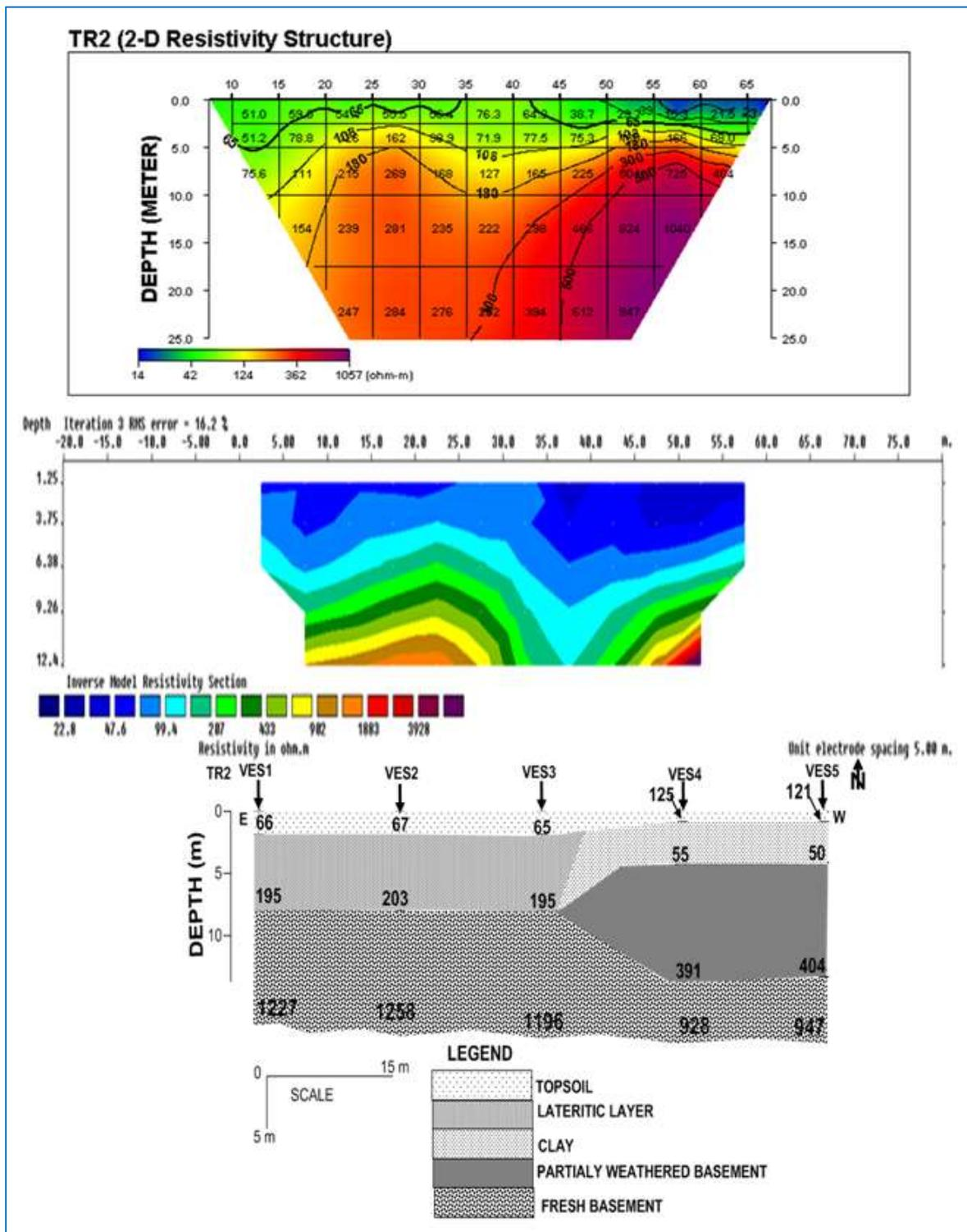
Fig. 19. Correlation of 2D Dipole-Dipole Pseudosection, 2D Lateral Resistivity Imaging and Geoelectric Section along Traverse Two
