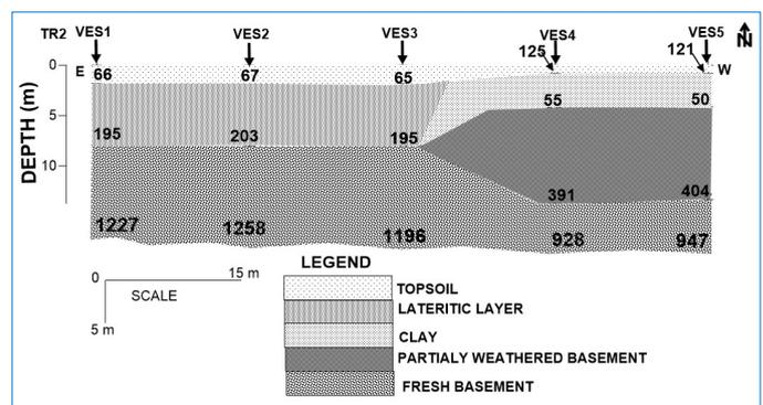
Fig. 13. Geoelectric section along Traverse Two
