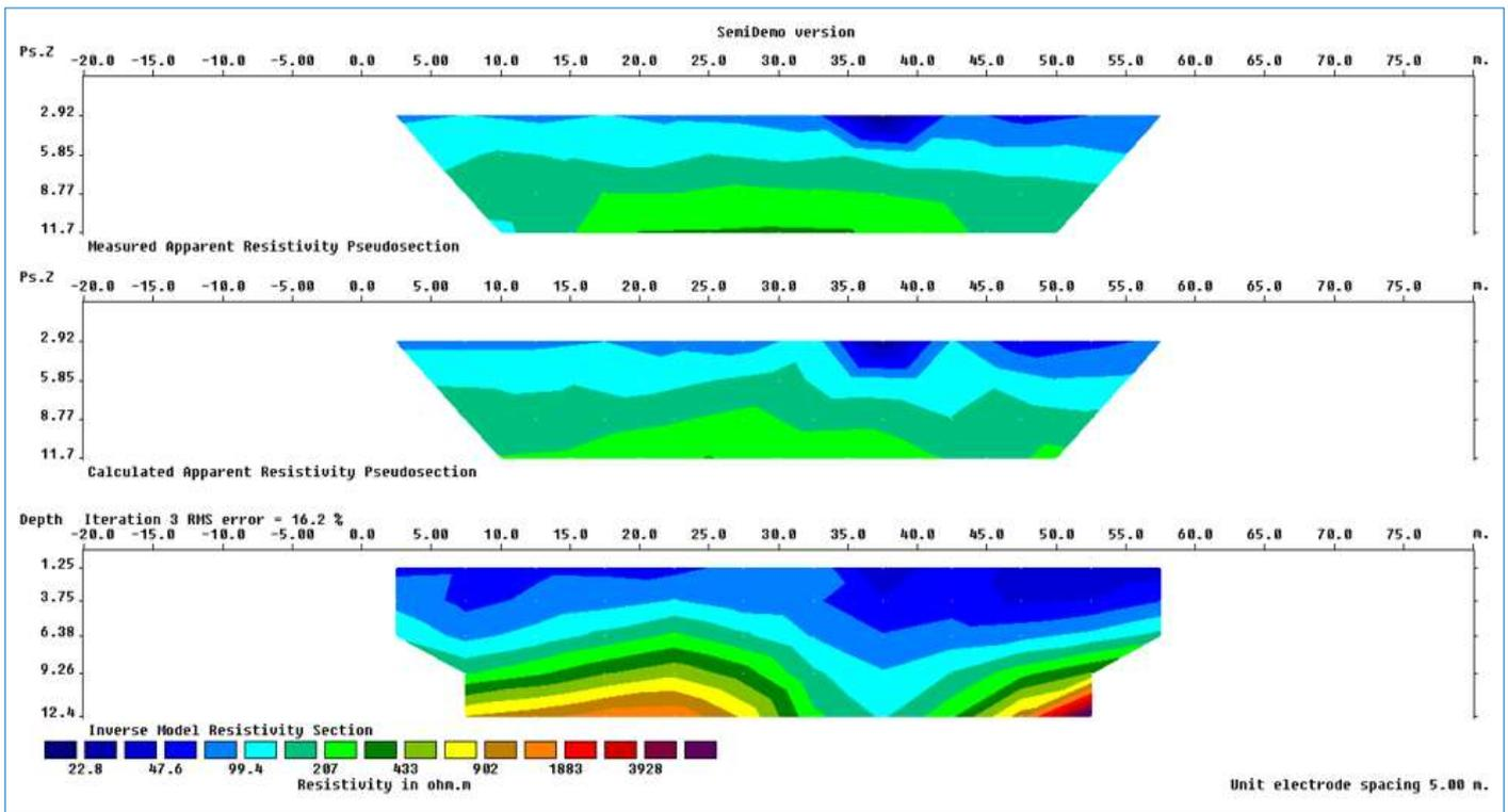
Fig. 10. Lateral Resistivity Profiling along Traverse Two
