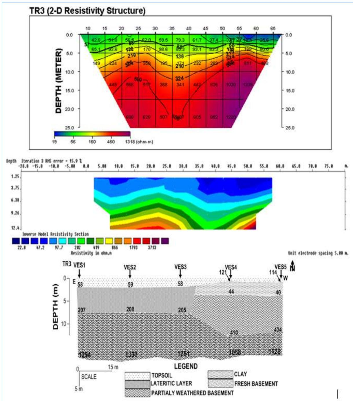
Fig. 20. Correlation of 2D Dipole-Dipole Pseudosection, 2D Lateral Resistivity Imaging and Geoelectric Section along Traverse Three
