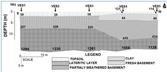
Fig. 14. Geoelectric section along Traverse Two
