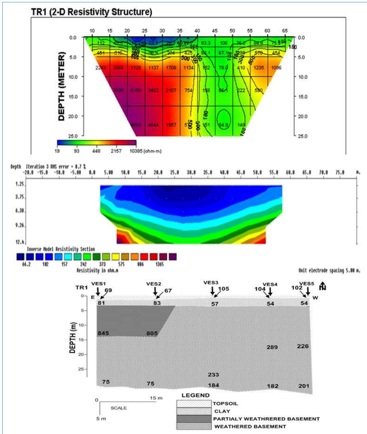
Fig. 18. Correlation of 2D Dipole-Dipole Pseudosection, 2D Lateral Resistivity Imaging and Geoelectric Section along Traverse One
