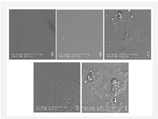
Fig. 1. SEM images of the ceramic surfaces (x 4000); A. Control (No treatment), B. 10% CP, C. 15% CP, D. 20% CP, and E. 35% CP gel was applied
