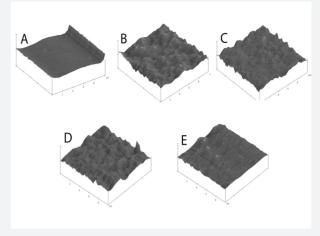
Fig. 2. Typical AFM images of the ceramic surfaces: A. Control (No treatment), B. 10% CP, C. 15% CP, D. 20% CP, and E. 35% CP gel was applied.
