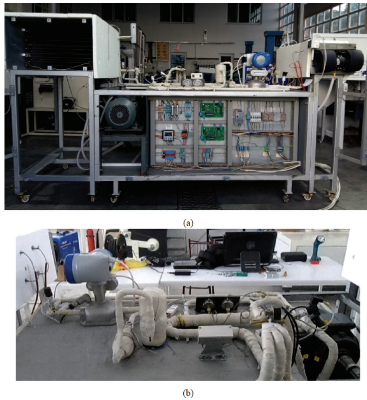
Figure 2. Photographs of the experimental AAC system; (a) Front view, (b) Rear view.
