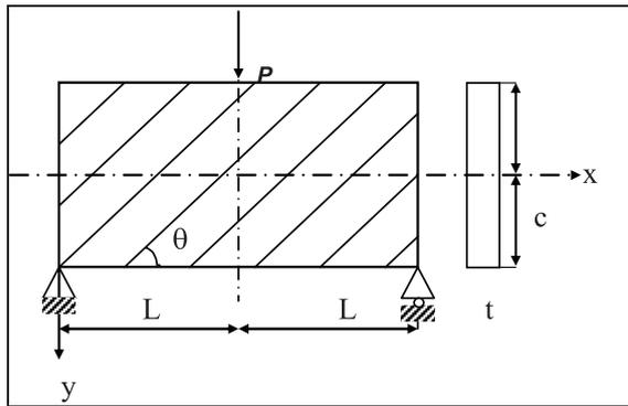
Figure 1. Simply supported composite beam under a single force.
