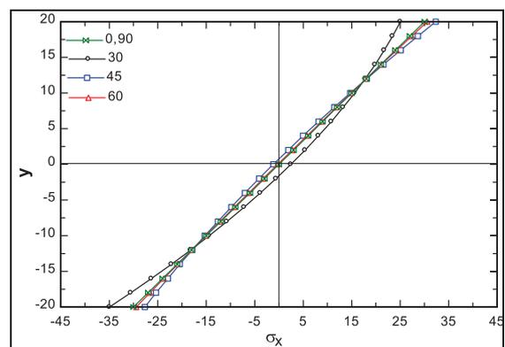
**Figure 2. Normal stresses ( $\sigma_x$ ) with respect to different orientation angles ((a)  $x=80$  mm, (b)  $x=0$  mm).**
