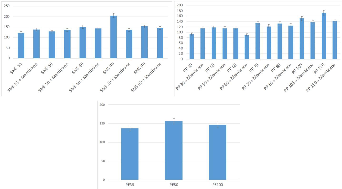
Figure 5. Thermal absorption of the samples ( $W.s^{1/2}/m^2.K$ )
