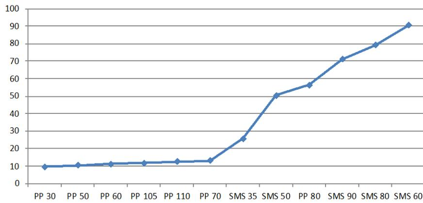
**Figure 9.** Water penetration resistance results for front side of SMS and PP samples (Pa)
