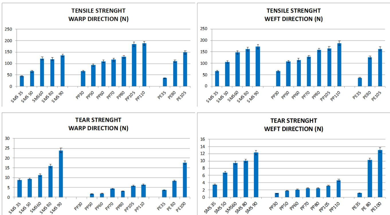
**Figure 1.** Tensile and tear strength of nonwoven fabrics
