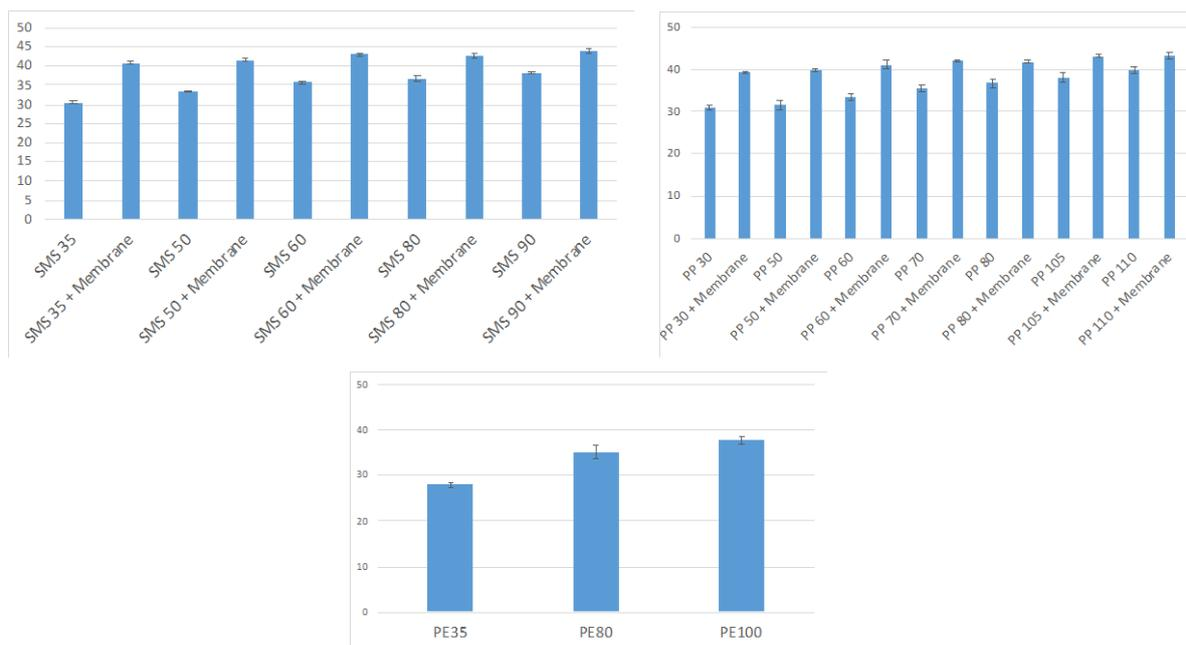
Figure 2. Thermal conductivity of the samples in (mW/m.K)
