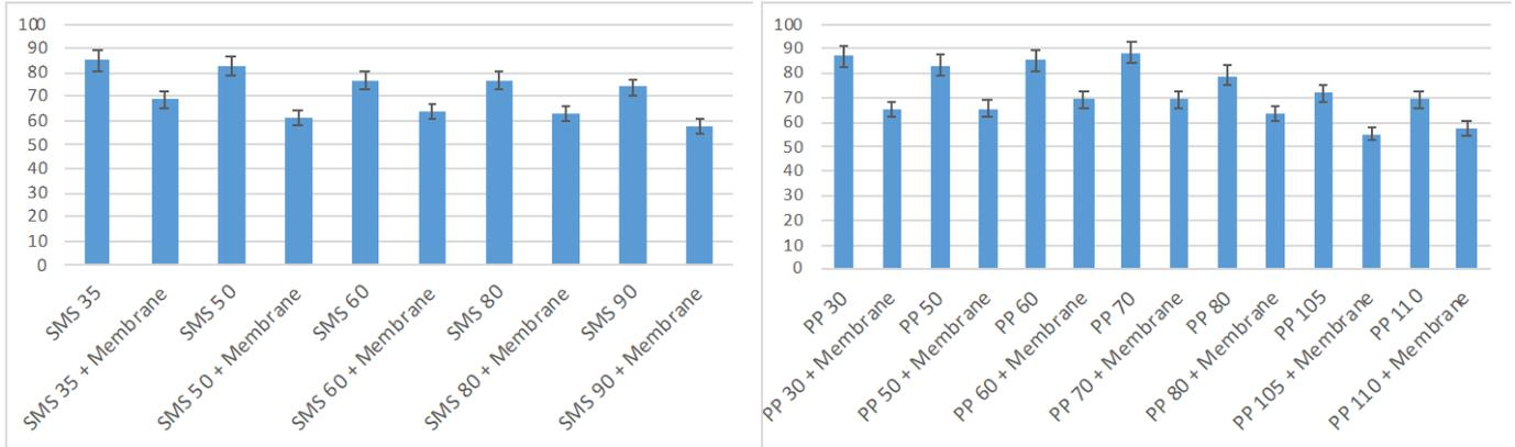
Figure 7. Relative water vapour permeability of the samples (%)
