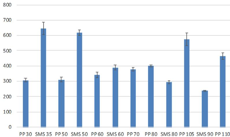
Figure 8. Air permeability test results (L/m<sup>2</sup>/sec)
