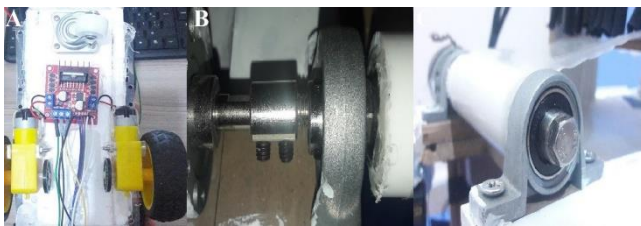
Figure 2 a) Positions of Motor and Driver in the process b) Coupling Connection to Motor Shaft c) Conveyor Belt Bearing.
