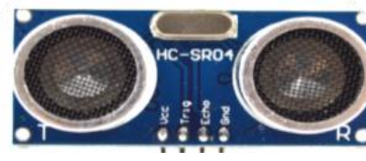
Figure 4. HCSR-04 Ultrasonic Sensor.
