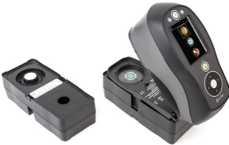
Figure 1. Calibration plate and X-Rite Ci60 portable spectrometer.
