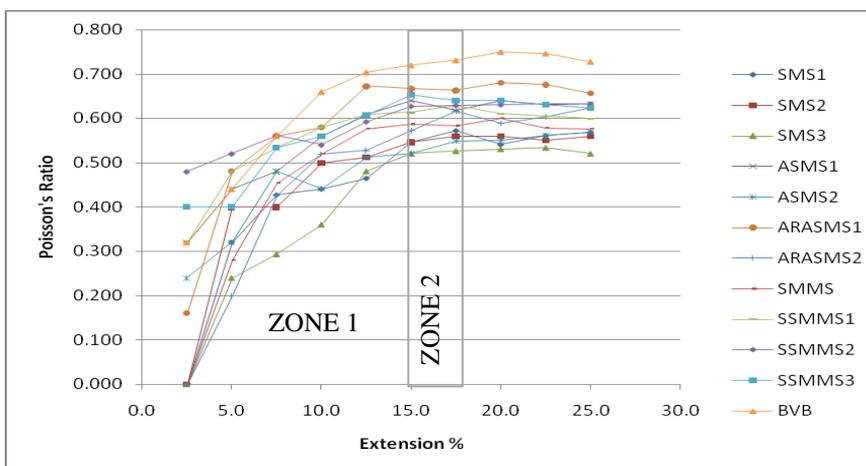
Figure 6. Poisson's ratio values of the non-woven fabrics in Cross Direction
