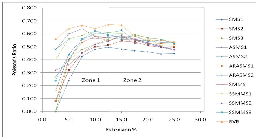
Figure 5. Poisson's ratio values of the non-woven fabrics in Machine Direction
