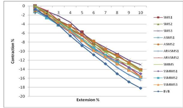
Figure 4. Spatial deformation of the fabric in the Cross Direction
