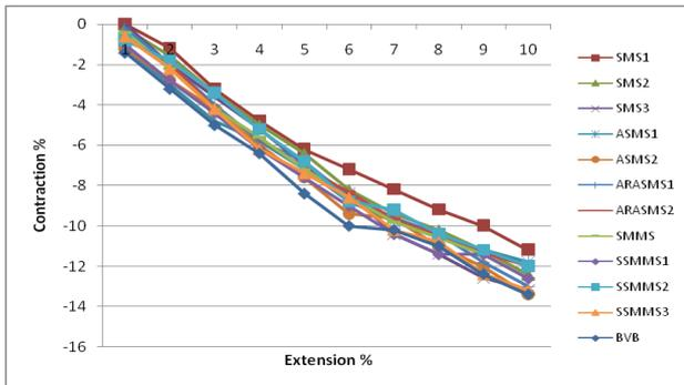
Figure 3. Spatial deformation of the fabric in the machine direction
