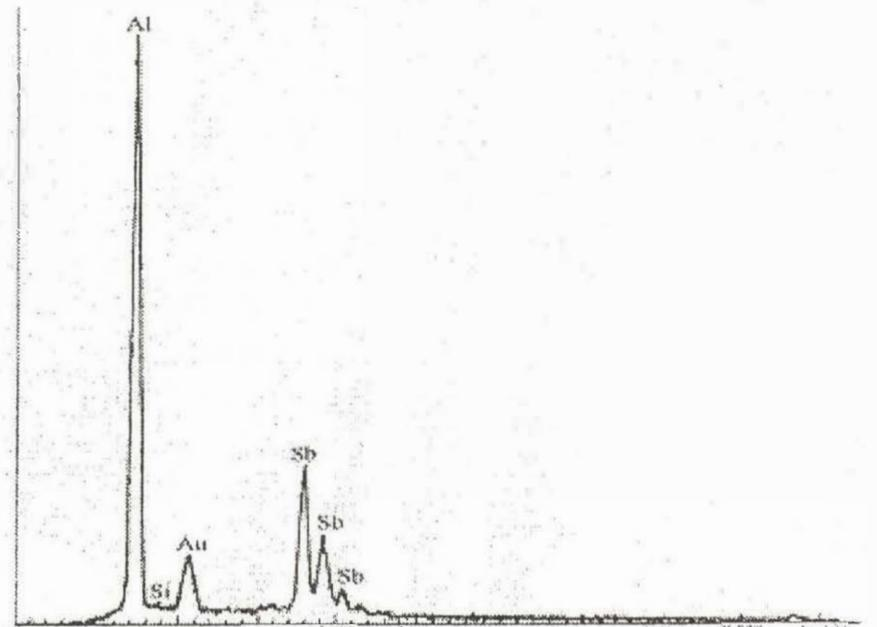
Figure 9. Energy dispersive X-ray spectra recorded from 1 %Sb added Al-12.5% Si alloy.
