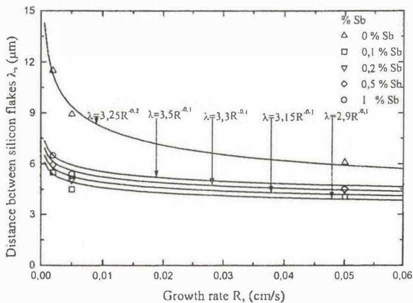
Figure 7. The relation between growth rate and distance between interflakes
