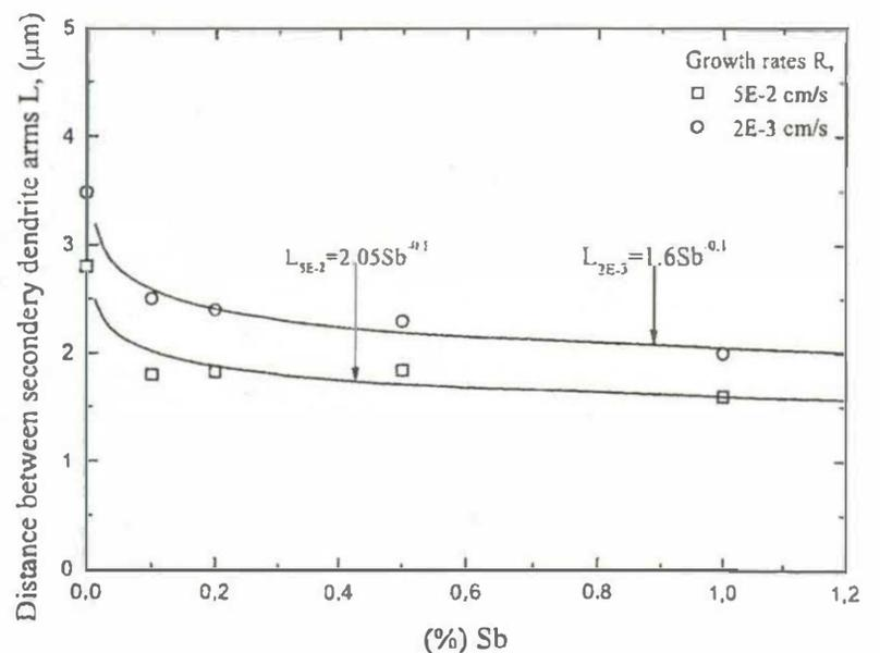
Figure 3. Change in the distance of secondary dendrite arms due to increase in Sb amount in the alloy
