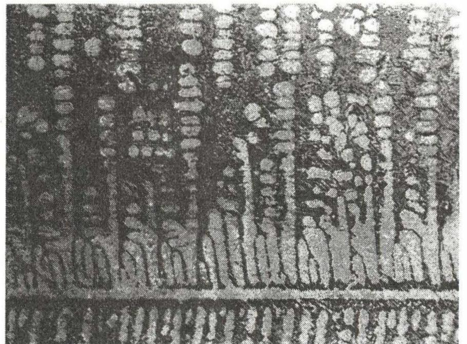
Figure 2. The effect of 0.1 % Sb addition on the formation of dendritic  $\alpha$ -Al phase (X 100)
