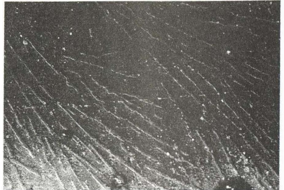
Figure 5. The effect of Sb addition on the eutectic morphology (a: 0 % Sb, b: 0.1 % Sb) (X2000)
