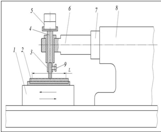
**Figure 2.** Installation diagram for determining the cutting ability of diamond honing stones: 1 – slide; 2 – diamond bar; 3 – processed sample; 4- rack; 5 – loads; 6 – mandrel; 7 – movable sleeve; 8 – tailstock; 9 – screw stop; L – length of the sliding path on the abrasive surface.
