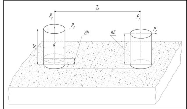
**Figure 1.** Scheme for determining the cutting ability of a diamond bar at processing of various materials:  $P_y$  – radial cutting force, MPa;  $P_z$  – tangential cutting force, MPa;  $d$  – diameter of the test material sample, mm;  $h_1$  and  $h_2$  – sample height, respectively, before and after processing, mm;  $\Delta h$  – the amount of linear material removal, mm;  $L$  – length of the path traversed by the sample on the abrasive surface, mm.
