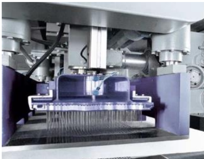
Figure 1: Needle punching machine as a MMD.
