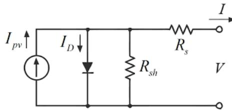
Figure 2. Photovoltaic module equivalent circuit.
