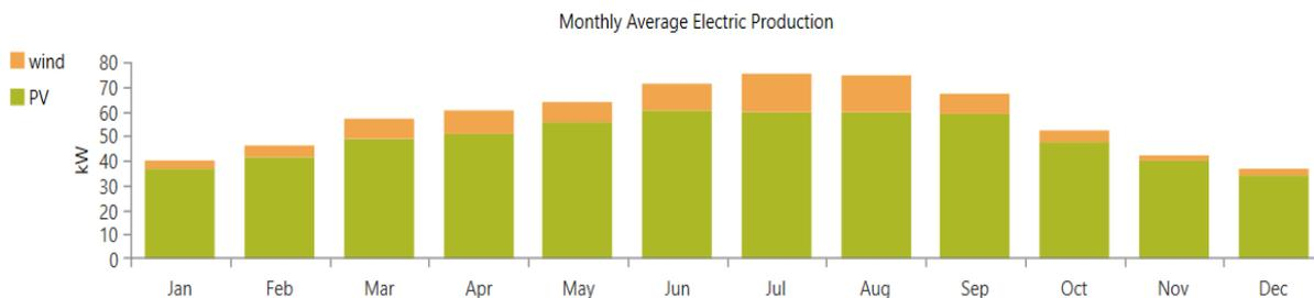
Figure 4. Power generation by PV and wind turbine in HWS system.
