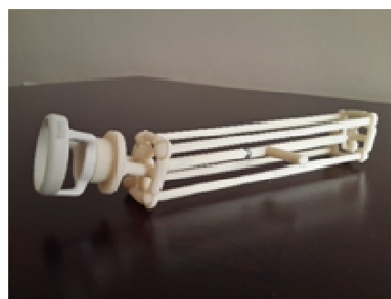
Figure 3. Rapid prototyped parallel manipulator
