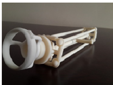
Figure 3. Rapid prototyped parallel manipulator
