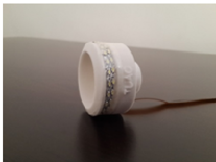
Figure 5. Rapid prototyped, LED illumination system integrated cervicovaginal cap
