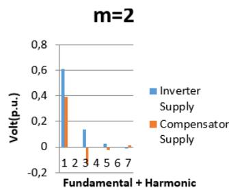
Figure 26. Fundamental and harmonics supply by inverter and filter (1<sup>st</sup>, 3<sup>rd</sup>, 5<sup>th</sup>, and 7<sup>th</sup>) at  $m = 2.0$ .
