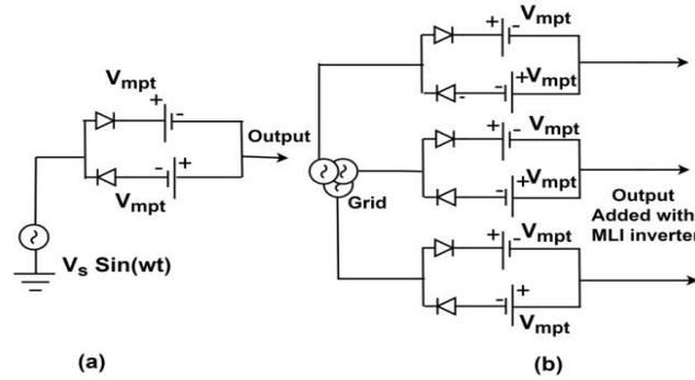
Figure 4. (a) Single, (b) three phase clamper circuits.
