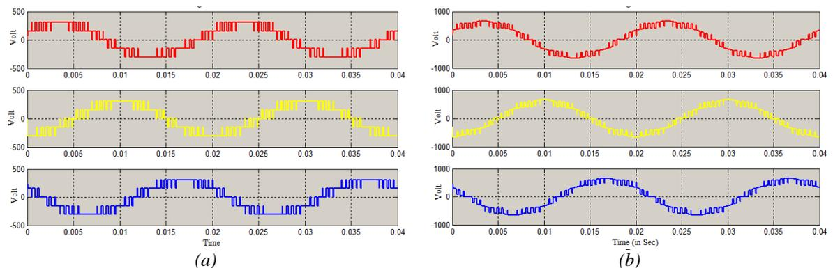
Figure 23. Final output at  $m=2.0$ : (a) without filter, (b) with filter.
