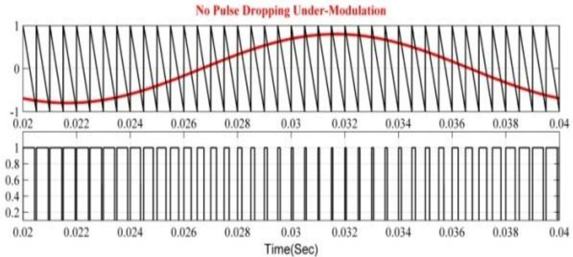
Figure 3. No-pulse dropping in under modulation.
