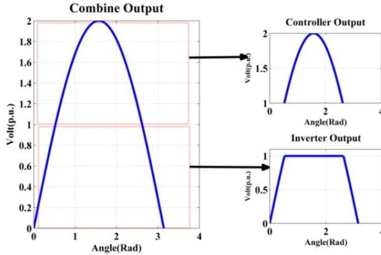
Figure 7. Filter and inverter output waveform.
