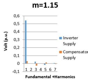
Figure 24. Fundamental and harmonics supply by inverter and filter (1<sup>st</sup>, 3<sup>rd</sup>, 5<sup>th</sup>, and 7<sup>th</sup>) at  $m = 1.15$ .
