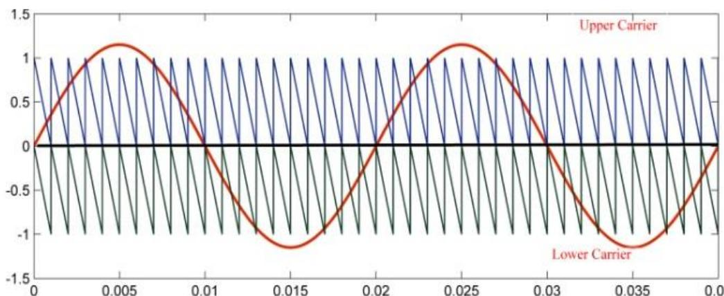
Figure 10. Carrier wave for NPC
