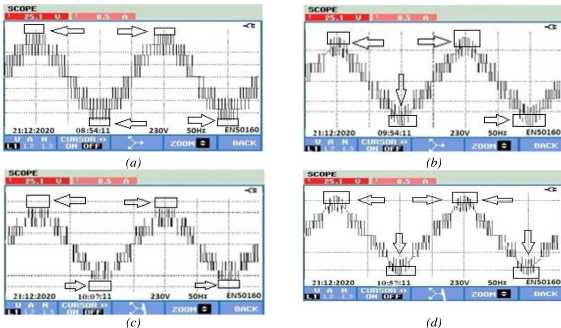
Figure 29. (a) Overall output at  $m=1.5$  without stabilizer, (b) experimental validation of Fig. 22 with stabilizer, (c) overall output at  $m=2$  without stabilizer, and (d) experimental validation of Fig. 23 with stabilizer.
