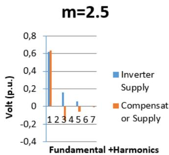
Figure 27. Fundamental and harmonics supply by inverter and filter (1<sup>st</sup>, 3<sup>rd</sup>, 5<sup>th</sup>, and 7<sup>th</sup>) at  $m = 2.5$ .
