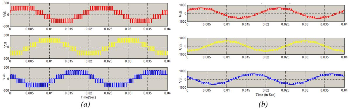
Figure 21. Final output at  $m=1.15$ : (a) without filter, (b) with filter.
