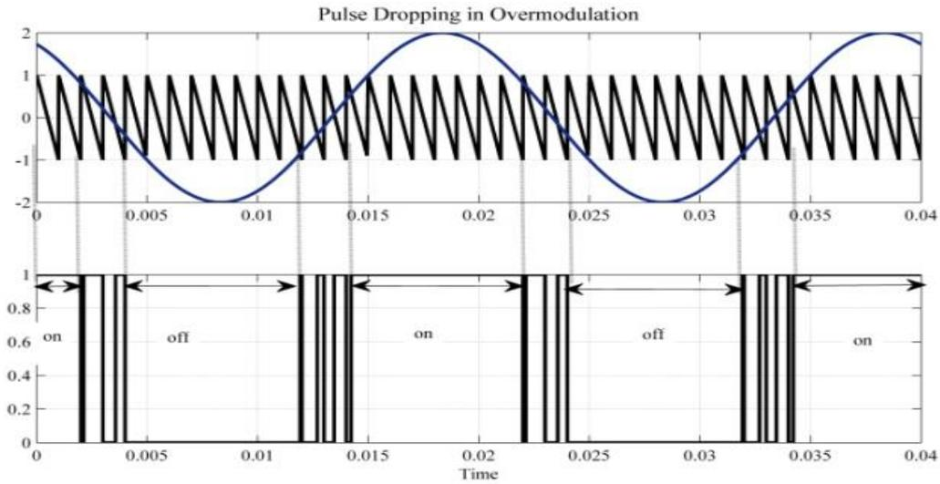
Figure 2. Pulse dropping in over-modulation.
