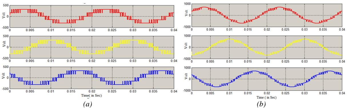
Figure 22. Final output at  $m=1.5$ : (a) without filter, (b) with filter.
