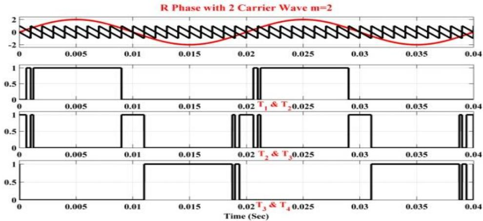
Figure 13. R phase with the combined switching pairs ( $T_1 T_2$ ,  $T_2 T_3$ , and  $T_3, T_4$ ) at  $m=2.0$ .
