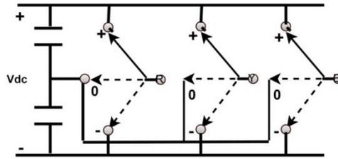
Figure 8. Multi-level inverter with single pole triple throw
