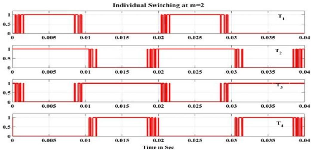
Figure 14. Switching pulses for R phase switches at  $m=2.0$ .
