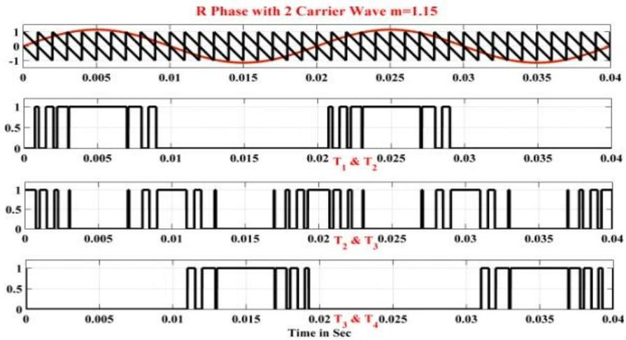
Figure 11. R phase with combined switching pairs ( $T_1 T_2$ ,  $T_2 T_3$ , and  $T_3 T_4$ ) at  $m=1.15$ .
