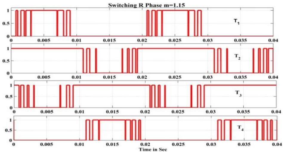
Figure 12. R Phase has individual Switching Pairs ( $T_1, T_2, T_3, T_4$ ) at  $m=1.15$ .
