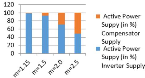
Figure 28. Inverter and filter contribution at various modulation indexes.
