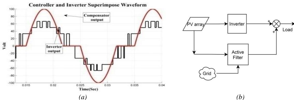
Figure 6. (a) Superimpose filter and inverter output voltages, (b) the block diagram.
