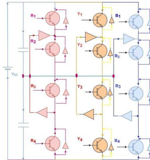
Figure9. Multi-level neutral point clamped inverter
