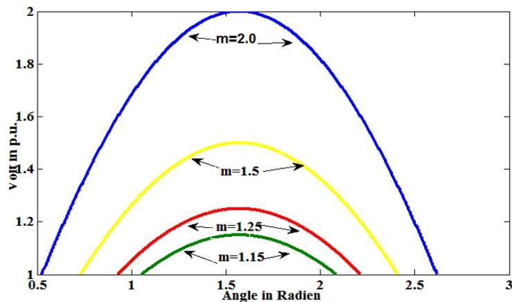
Figure 5. Filter output at various modulation indexes in half cycle.
