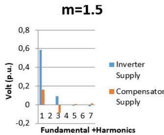
Figure 25. Fundamental and harmonics supply by inverter and filter (1<sup>st</sup>, 3<sup>rd</sup>, 5<sup>th</sup>, and 7<sup>th</sup>) at  $m = 1.5$ .
