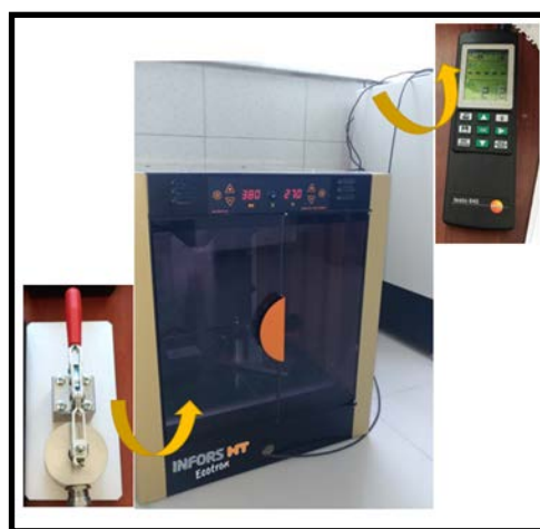
Figure 1. Measurement of water activity of hazelnuts with desired moisture levels under controlled temperature change.
