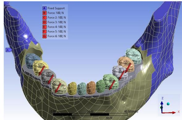
**Figure 3.** The view of implants, their loading locations and fixed support
