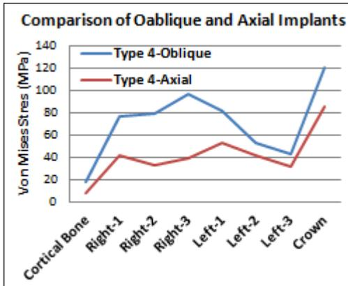
Figure 5. The comparison of stress values according to oblique and axial loading types
