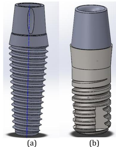
**Figure 1. a)** Short dental implant and **b)** regular dental implant model
