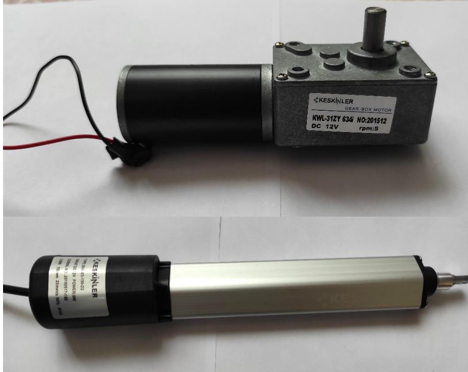
Figure 6. Geared DC motor (upper) and linear DC motor used in the solar tracking system
