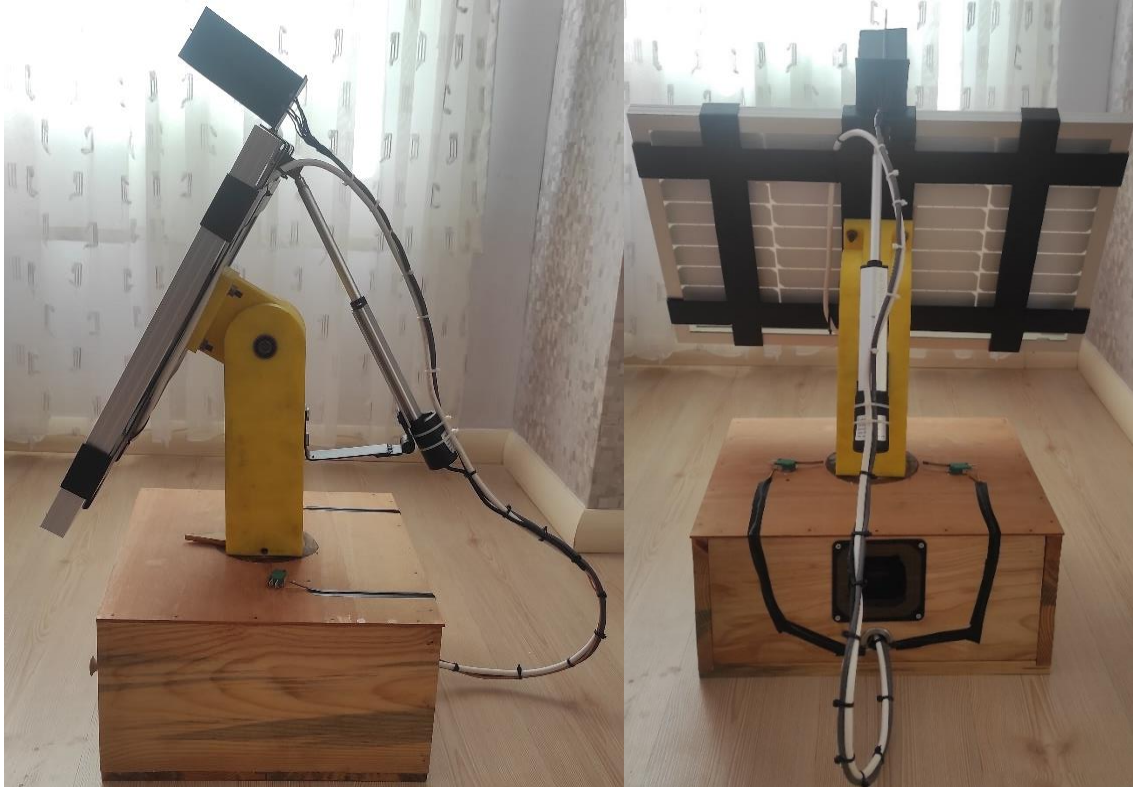
Figure 7. Final state of the solar tracking system
