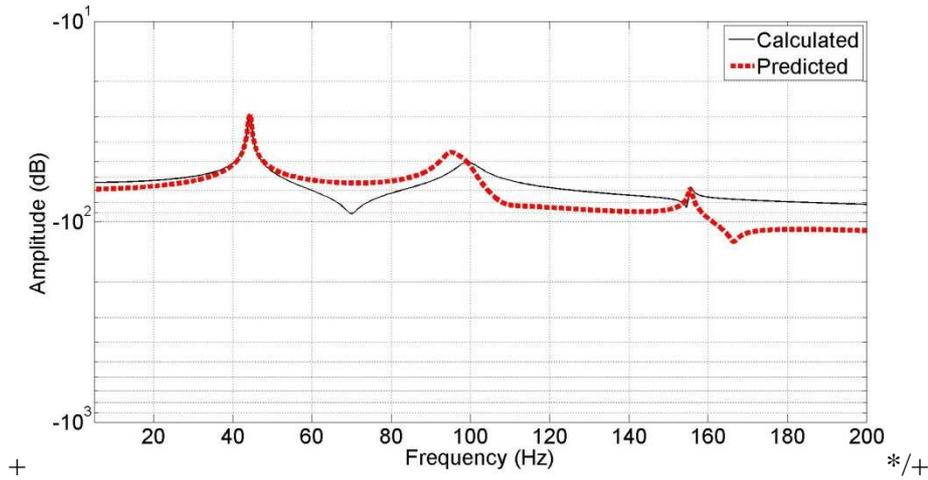
**Figure 4.** Vibration response,  $x_3$  (without considering  $f_3 = 20$  N)
