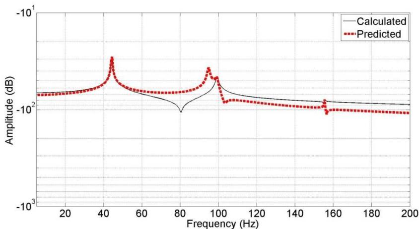
**Figure 3.** Vibration response,  $x_3$  (without considering  $f_3 = 10$  N)
