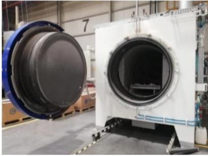
Figure 1. IPSEN Nitration Furnace
