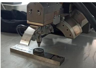
**Figure 3.** Residual Stress Measurement with XRD Method
