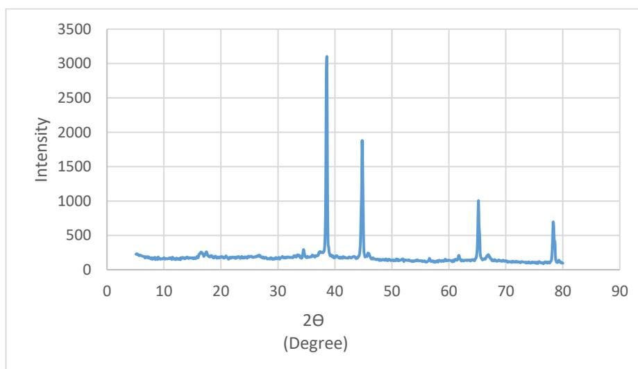
**Figure 3.** X-Ray Diffraction (XRD) pattern of  $\text{TiO}_2/\text{Al}_2\text{O}_3$  catalyst
