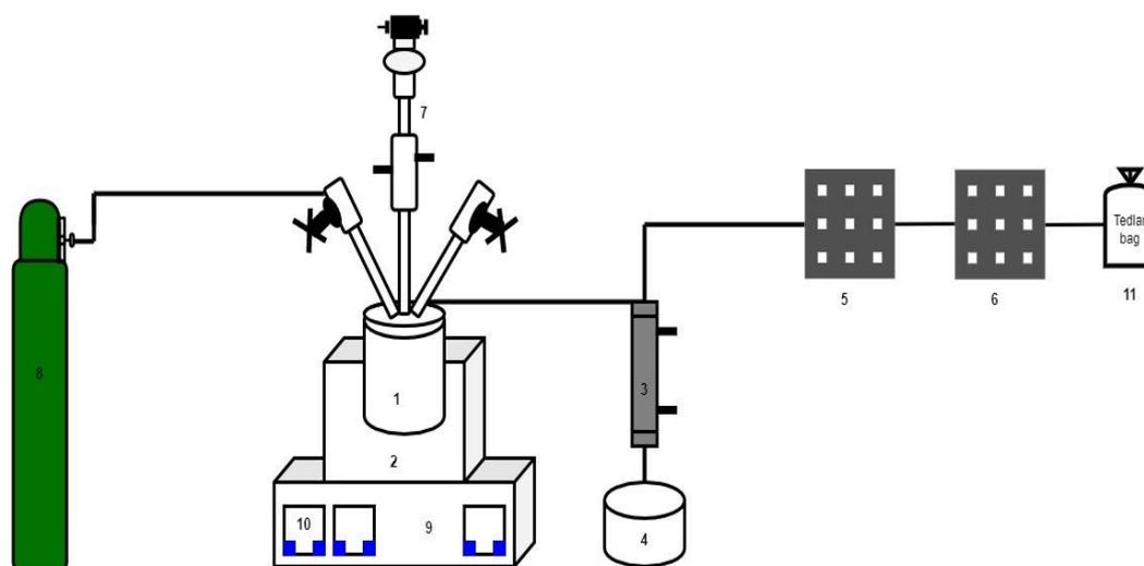
**Figure 1.** Schematic representation of the pyrolysis system 1- Reactor, 2- Tube furnace, 3-Liquid-gas phase separator, 4-Liquid product container, 5- Particle trap filter, 6-Moisture trap filter, 7-Thermo-couple, 8-Nitrogen tube, 9-Power supply, 10-Controller 11- Tedlar™ Bag
