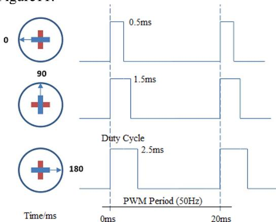
Figure 11. The duty-cycles of the square control signal
