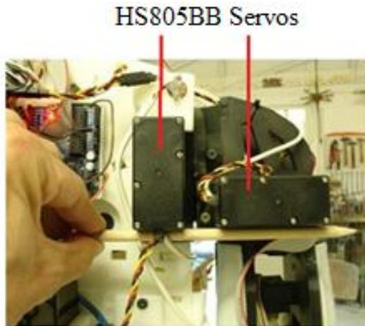
Figure 10. Shoulder joint of the humanoid robot [21]
