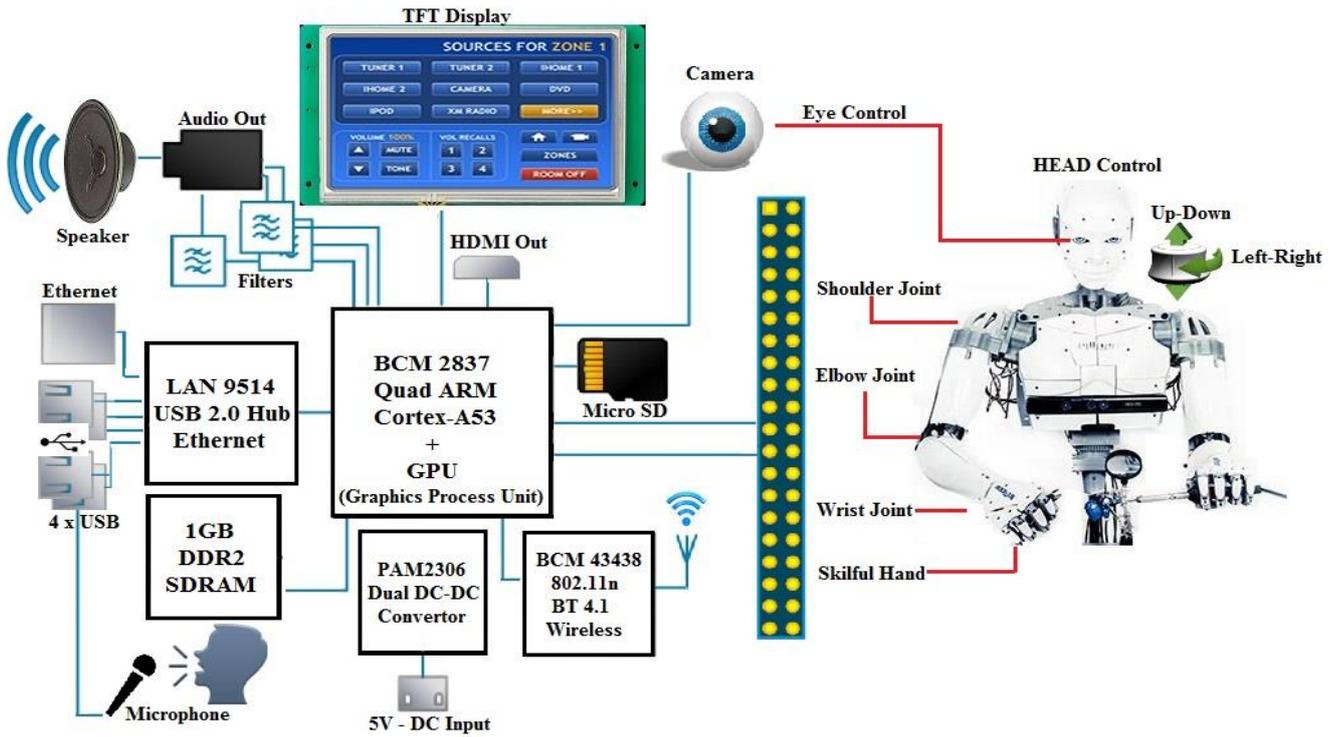
Figure 12. Connection of humanoid robot to peripherals
