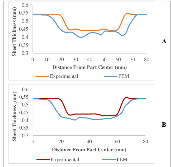
Fig. 4. Thickness comparisons. A) 8th experiment. B) 12th experiment.
