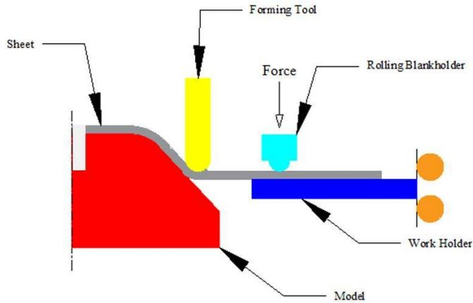
Fig. 1. Rolling blank holder method (TPIF-RL method) [10].
