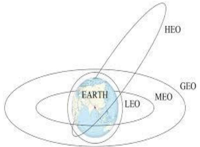
**Figure 3.** Orbit altitudes[3] LEO satellites are confined between 500 to 1500 km. altitude. The GEO satellite altitude is of around 36,000 km, MEO satellites altitude is in the range of 10,000 to 15,000 km. and MEO and LEO satellites are referred to as Non-Geostationary Orbit (NGSO) satellites.
