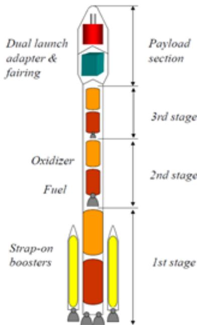
**Figure 1.** Three staged Rocket System [2]
