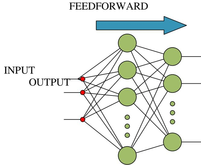
**Figure 1. Architecture of Backpropagation Multilayer Perceptron Model**
