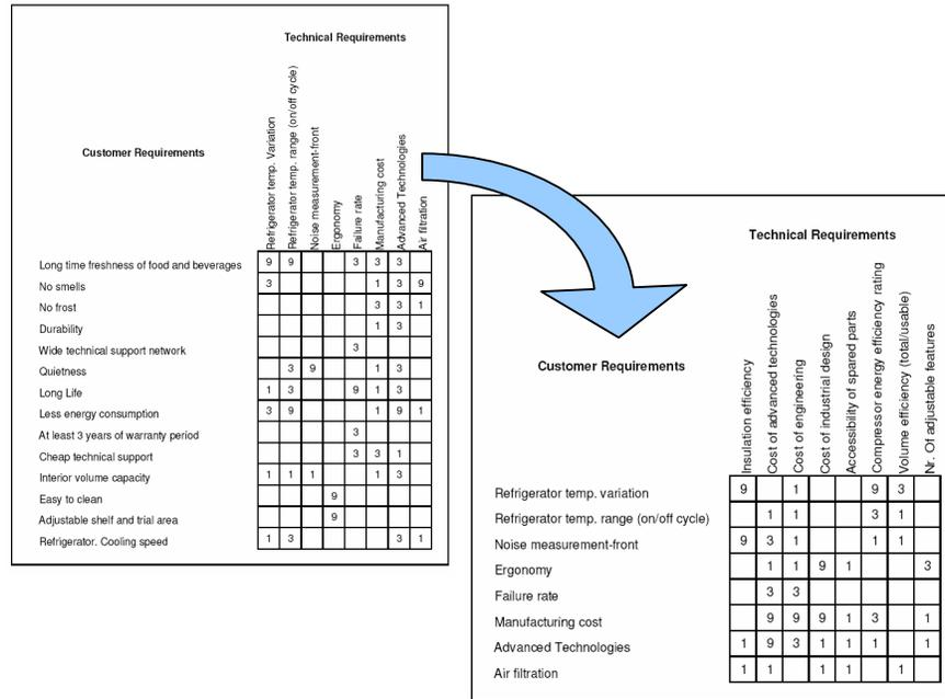
**Figure 5. HOWS and WHATS of the First 2 Phases of QFD**
