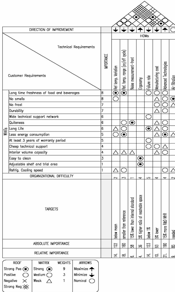
Figure 6. HOQ in the First Phase of QFD
