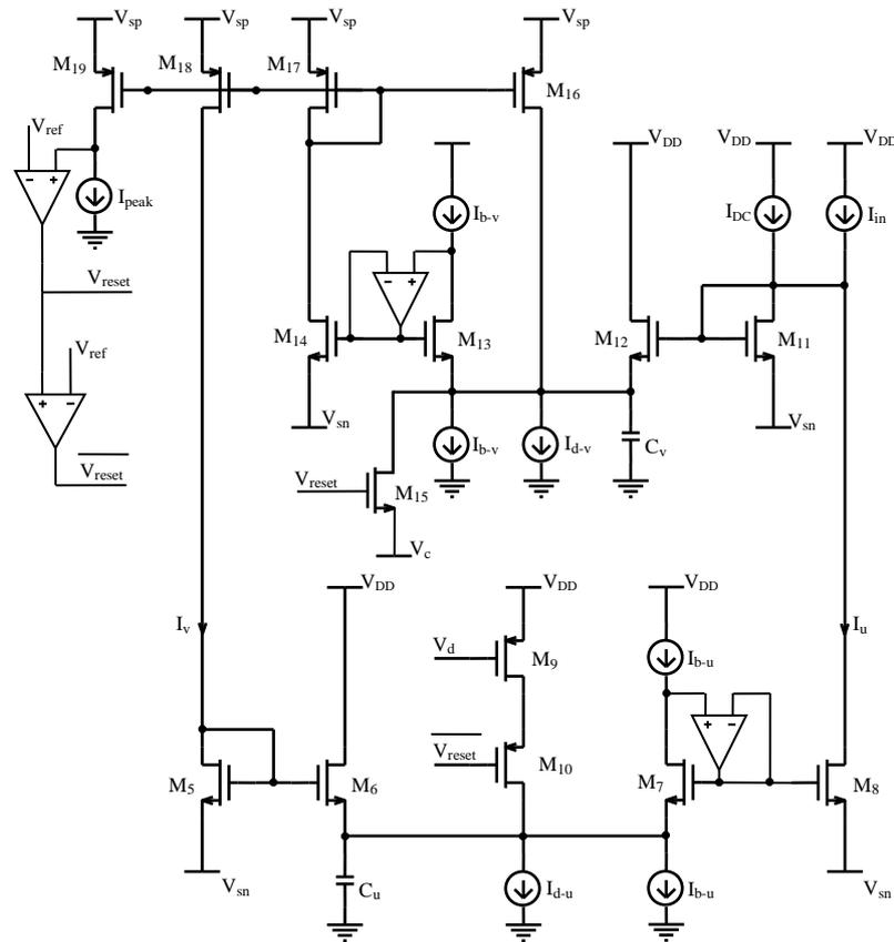
**Figure 2.** The overall neuron circuit.
