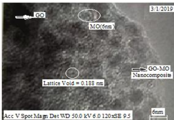
Figure 5. HR-TEM images of graphene oxide, manganese oxide and graphene oxide-manganese oxide nanocomposite
