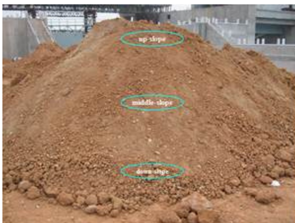
Figure 3. Positions to collect soil samples
