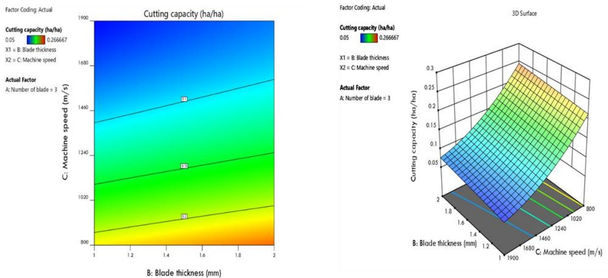
**Figure 12.** Contour and 3D surface plot of the cutting capacity at different machine speeds and blade thickness.
