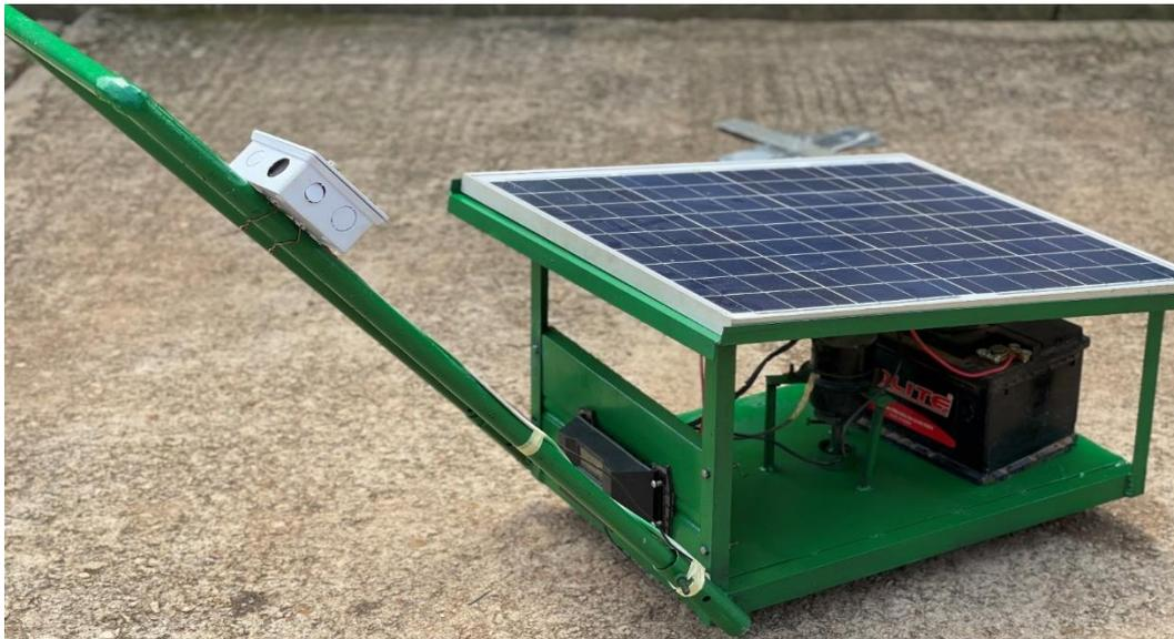
**Figure 3.** Assembled lawn mower.
