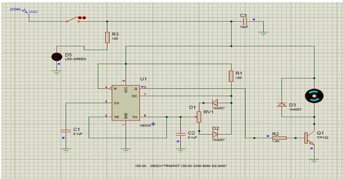
**Figure 4.** Circuit design of the speed controller.
