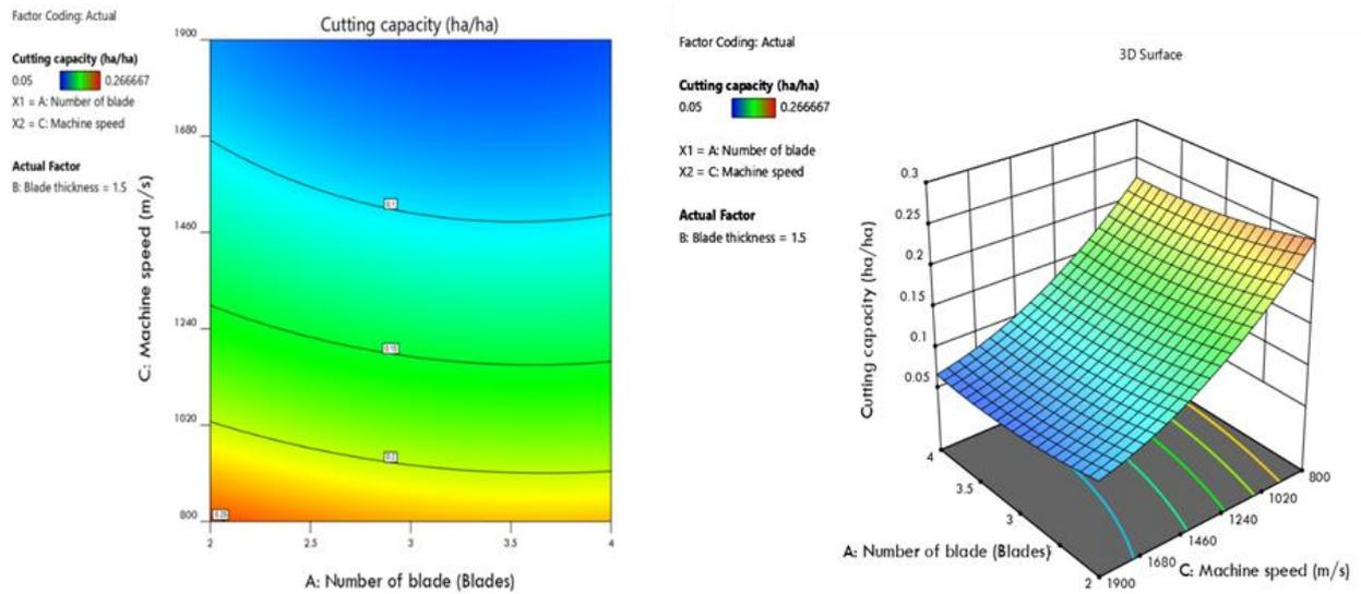
**Figure 11.** Contour and 3D surface plot of the cutting capacity at different machine speeds and number of blades.
