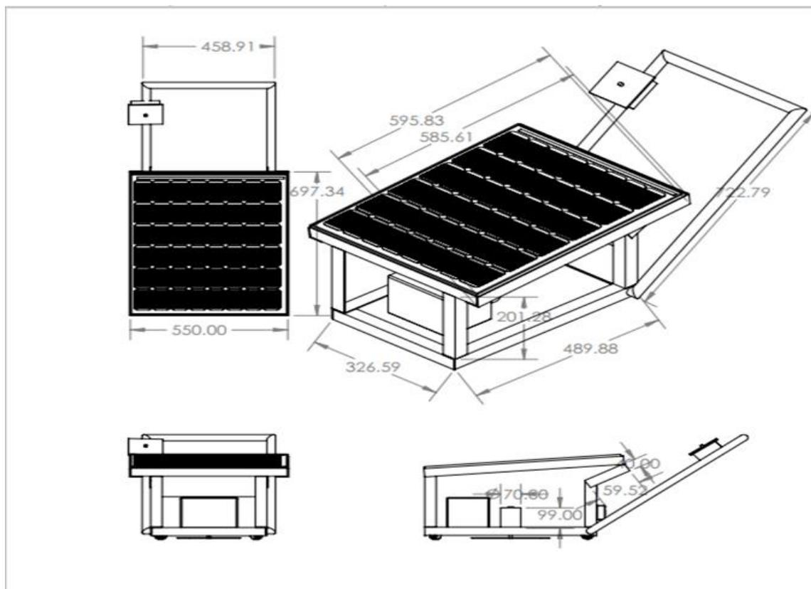
**Figure 2.** Orthogonal view of the designed lawn mower.
