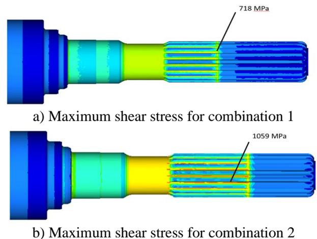
Figure 4 The maximum shear stress on the pitch diameter of the spline as a result of FEA
