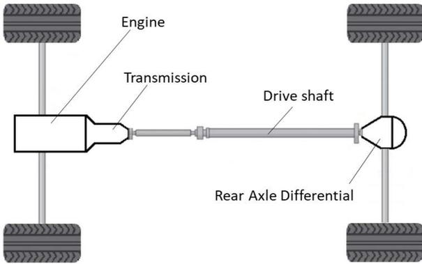
Figure 1 A classical driveline for the motor vehicle [2]
