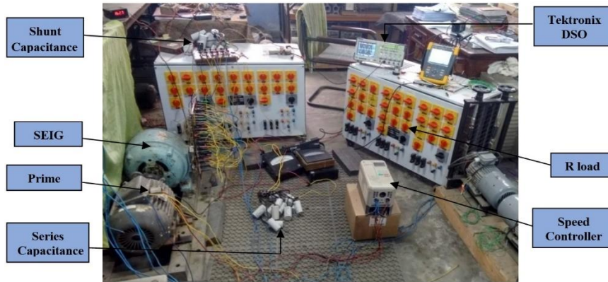
Figure 7. Illustration of three-phase short shunt SEIG test rig.
