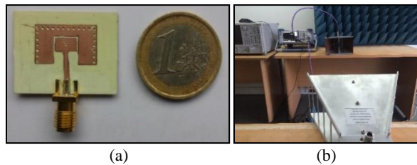
Figure 3. (a) Fabricated antenna (b) Measurement setup [22].
