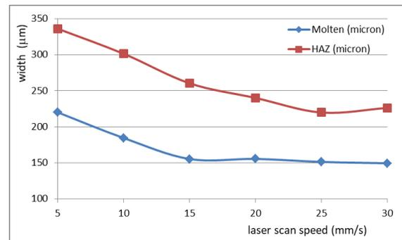
**Figure 2.** As can be seen from the change graph, the width of the molten region decreased linearly up to a scanning speed of 15 mm/s. At values above 15 mm/s, the width of the molten zone remained almost constant. The Violet-Brown heat tone line studied in this study decreased almost linearly up to a scan speed of 25 mm/s. After this value, the heat tone line remained almost constant as in the molten region.
