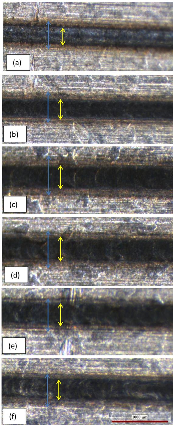
**Figure 1.** Optical microscope images and measurements of the grooves created with the CO<sub>2</sub> laser on dual-phase steel material with different scanning speeds. Scan speeds, (a) 5 mm/s , (b) 10 mm/s, (c) 15 mm/s, (d) 20 mm/s, (e) 25 mm/s, (f) 30 mm/s,
