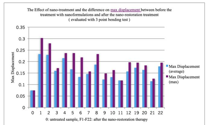
**Fig 4:** CNT/Ca(OH)<sub>2</sub> Nano-composites max-displacement data, evaluation by 3 point bending test, also effects of colloid stability on efficiency [20]
