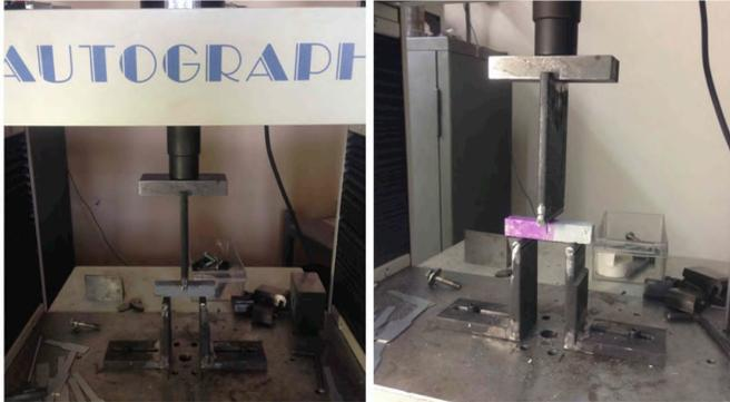
**Fig1 :** Destructive evaluation test, 3 Point bending test , to evaluate mechanical strength enhancement, [20]
