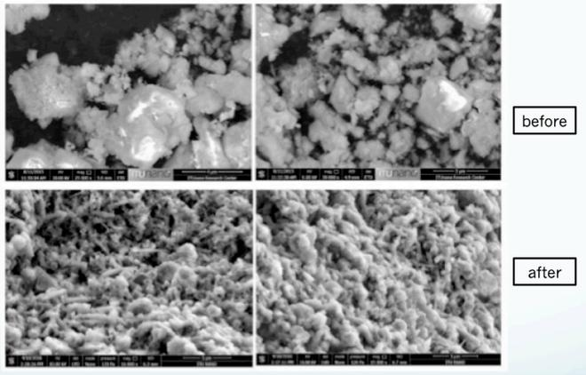
Fig 4: Evaluation of the Efficiency Criteria in nano-tech: SEM analysis of nano-composite treatment, all the defects has been consolidated with the nanoparticles has been shown. (before and after application) [20]
