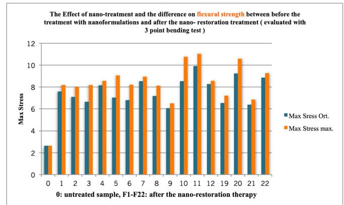
**Fig 3:** CNT/Ca(OH)<sub>2</sub> Nano-composites flexural strength evaluation by 3-point bending test, also effect of colloid stability and dispersion efficiency. [20]
