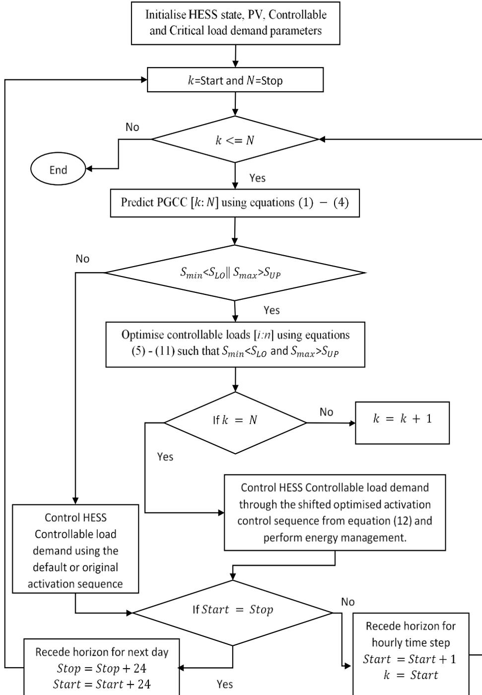
Figure 2. Flow chart for MPC Based on Adaptive PoPA for Load Shifting and Shedding algorithm
