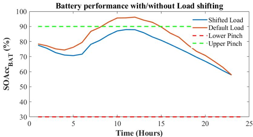
Figure 5. Original and shifted battery state of charge response in summer.
