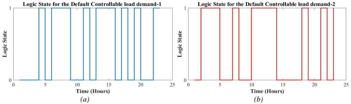
Figure 6. (a) Original logic state of the controllable load demand 1 in winter, (b) original logic state of the controllable load demand 2 in winter.
