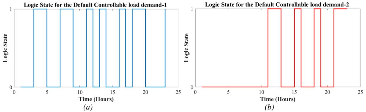
Figure 3. (a) Original logic state of the controllable load demand 1 in summer, (b) original Logic state of the shifted controllable load demand 2 in summer
