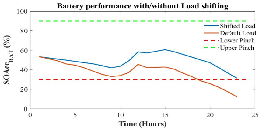
Figure 8. Original and shifted battery state of charge response in winter.
