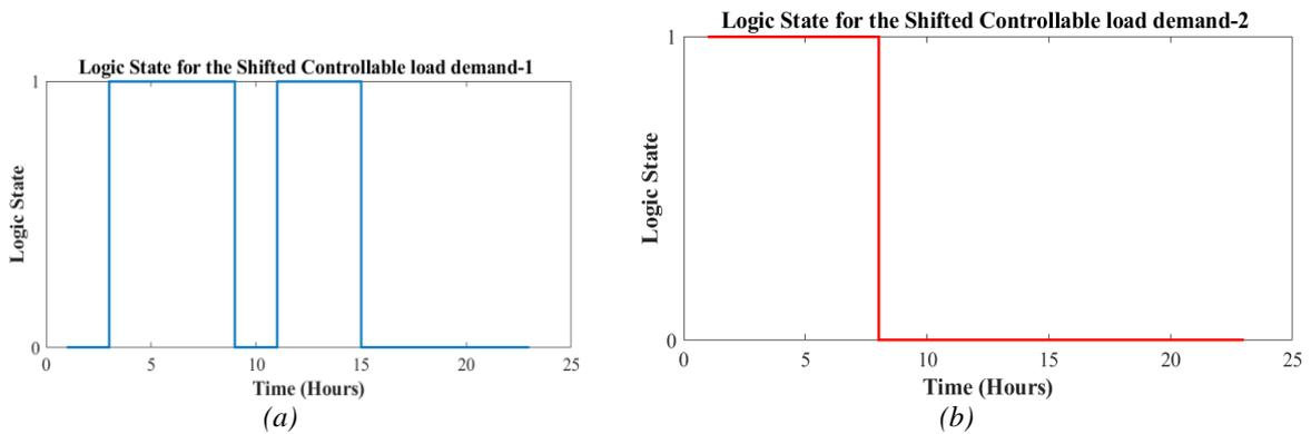
Figure 4. (a) Logic state of the shifted controllable load demand 1 in summer, (b) logic state of the shifted controllable load demand 2 in summer.
