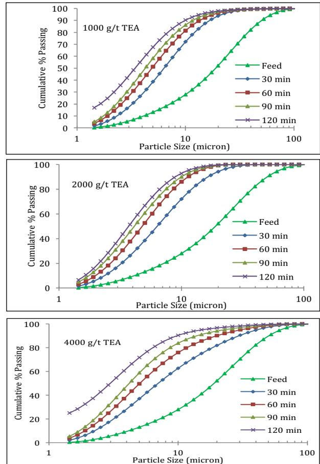
**Figure 2.** Particle size distribution data with TEA grinding
