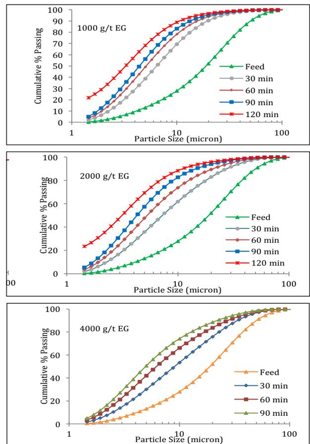
**Figure 3.** Particle size distribution data with EG grinding
