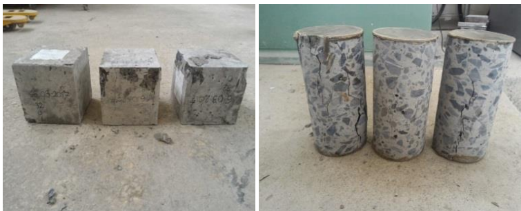
Figure 5. Cubes of 15 cm (left) and cores (right) on which compression test performed
