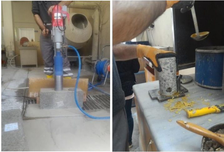
Figure 4. Coring process (left) and capping process (right)
