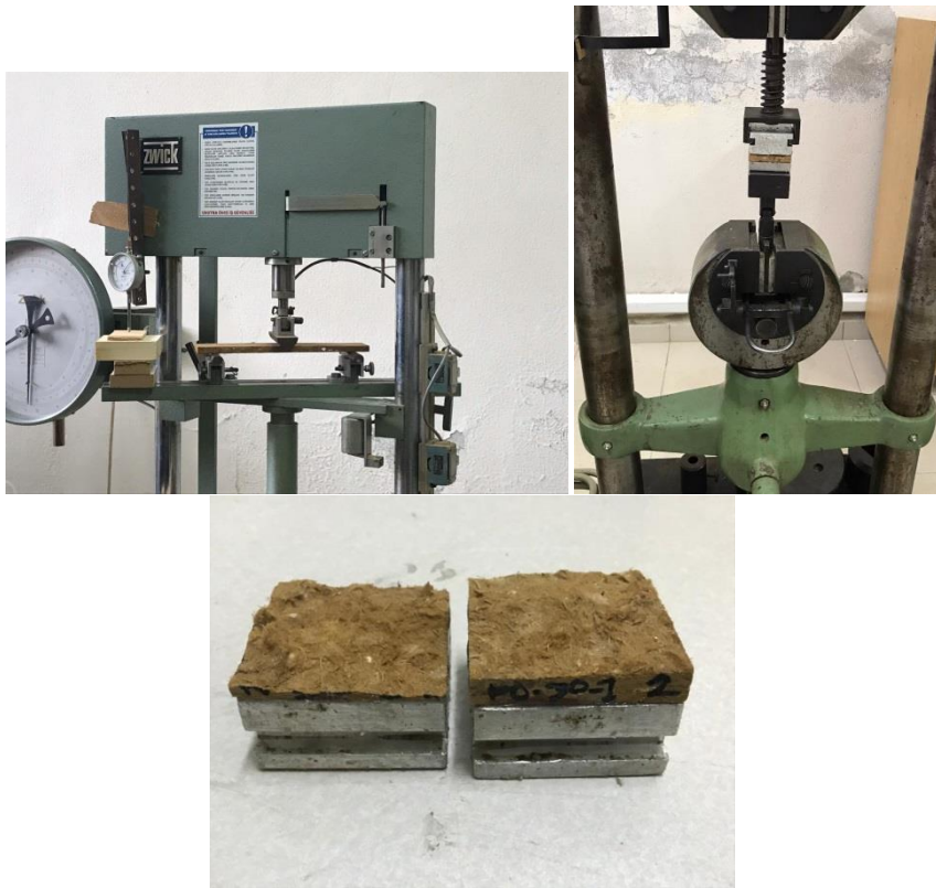
Figure 3. Mechanical tests of mycelium based MDF
