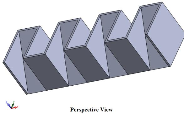
**Figure 2.** Inclined-bed rectangular weir.
