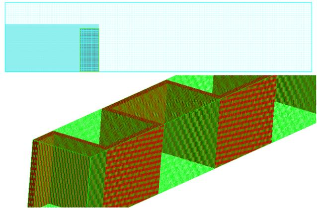
**Figure 4.** Rectangular labyrinth weir mesh structure.
