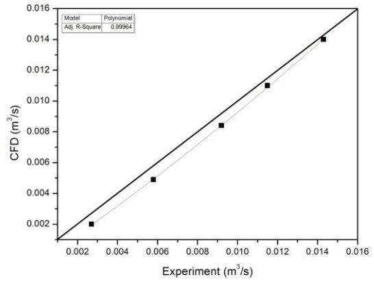
**Figure 20.** Comparison of inclined-bed rectangular weir discharge
