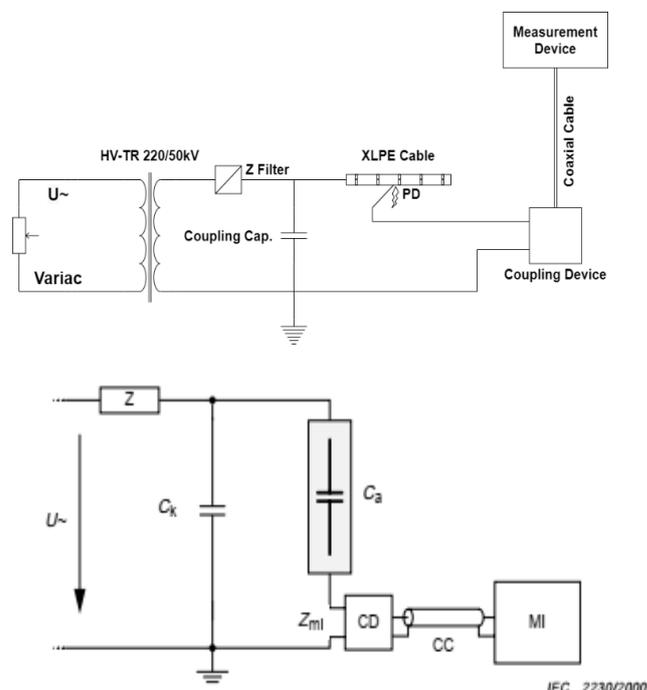
Figure 2. Circuit diagrams of the PD test system
