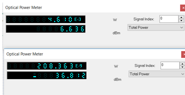
Figure 16. Optical powers of input and output signals measured in Watts and dBm for a fiber length of 70 km, for the hybrid WDM/TDM PON system
