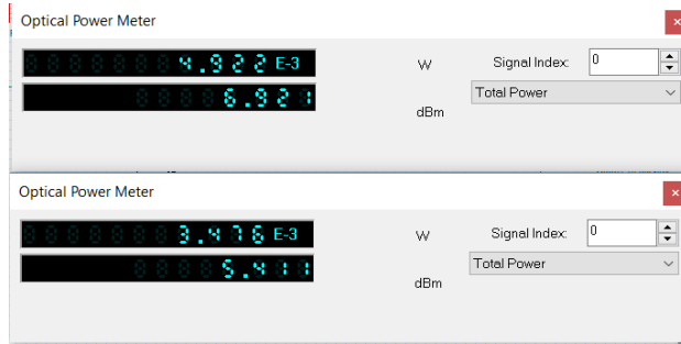
Figure 14. Optical powers of input and output signals measured in Watts and dBm for a fiber length of 10 km, for the hybrid WDM/TDM PON system
