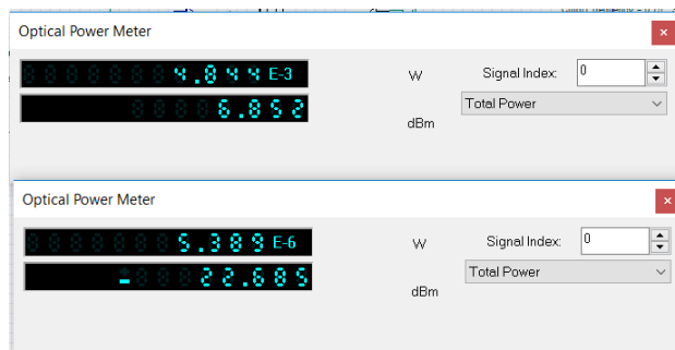
Figure 15. Optical powers of input and output signals measured in Watts and dBm for a fiber length of 50 km, for the hybrid WDM/TDM PON system
