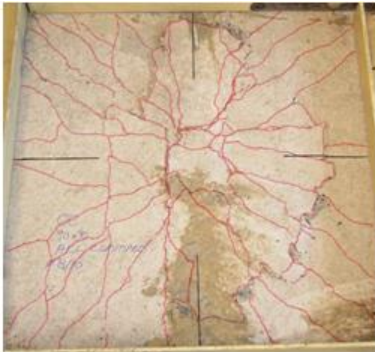
Figure 14. Failure pattern of AG4 slab
