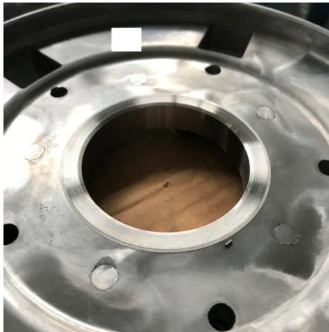
**Figure 10.** Precision turned part with pre-broaching hole
