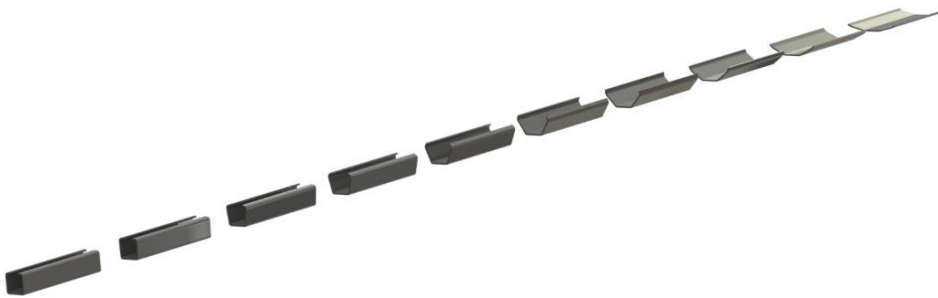
Figure 22. Solid models of the profiles at all stations
