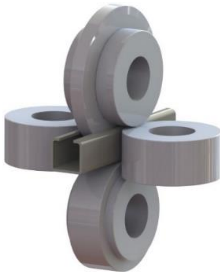
Figure 20. The profile and solid models of rolls at the L01 station
