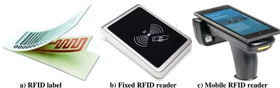
Figure 1. Most important elements of the RFID system
