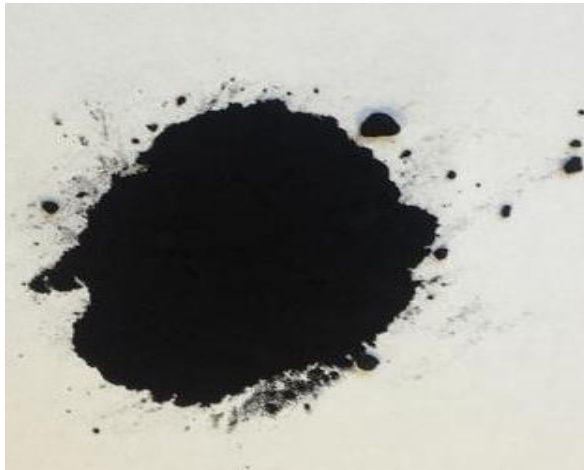
Figure 5. Copper oxide ( Cu_yO_x ) obtained after electrowinning.
