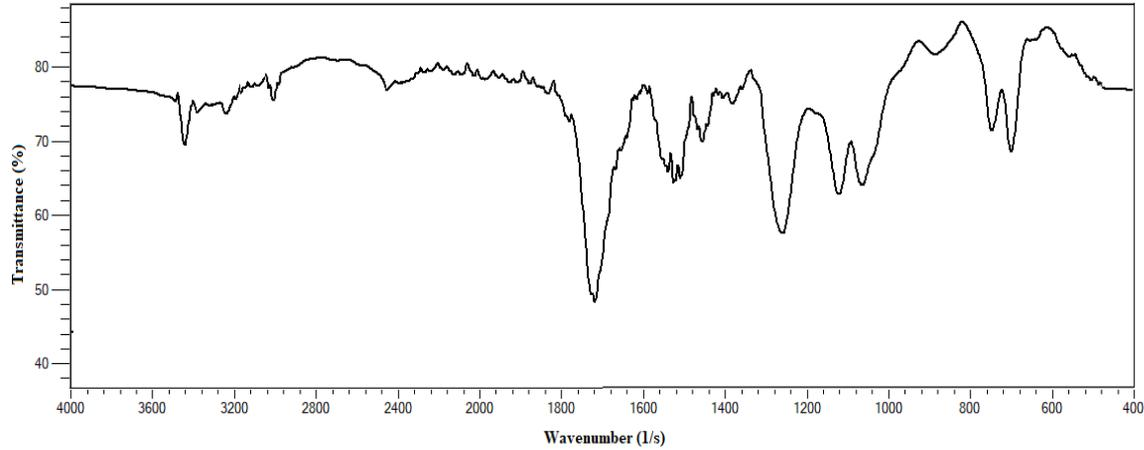
**Figure 5.** FTIR Spectra of WM Reinforced Polyester Composite for Experiment 3
