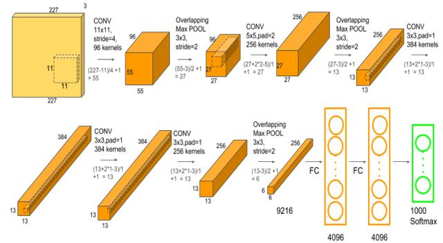
**Figure 6.** AlexNet architecture [18]
