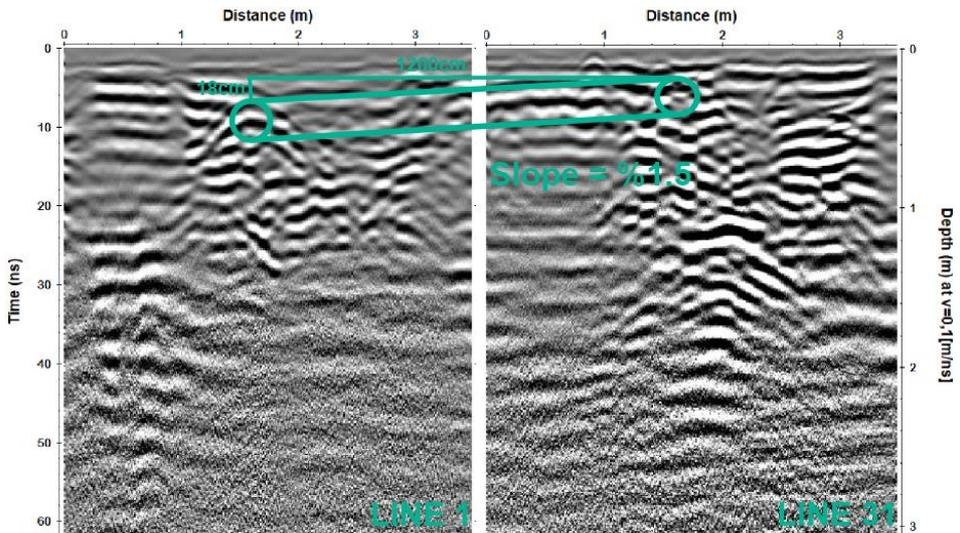
Figure 7. Slope image between line 1<sup>st</sup> and line 31<sup>st</sup> for study region 2.
